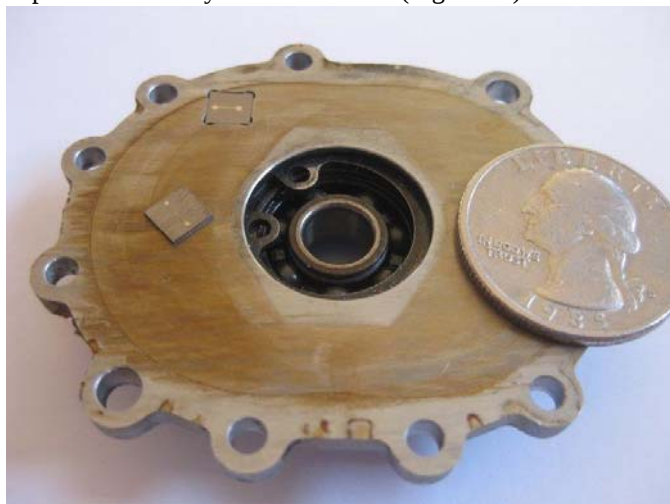
Figure 11: SiC temperature sensor embedded into near Top-Dead-Center position to control Carb-Smart.
