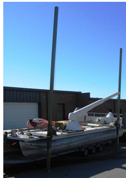
Figure 5-3: The spuds are shown deployed on the pontoon boat.
