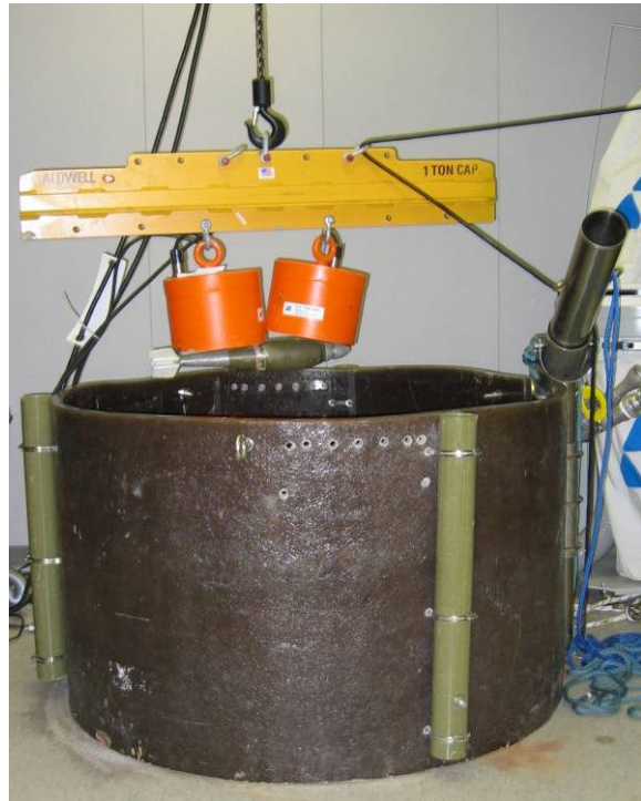
Figure 2-15. Electromagnet Recovery System lifting an 81mm mortar.
