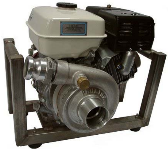
Figure 2-11. This image shows the centrifugal pump that is used to power the vacuum dredge and the water jet.
