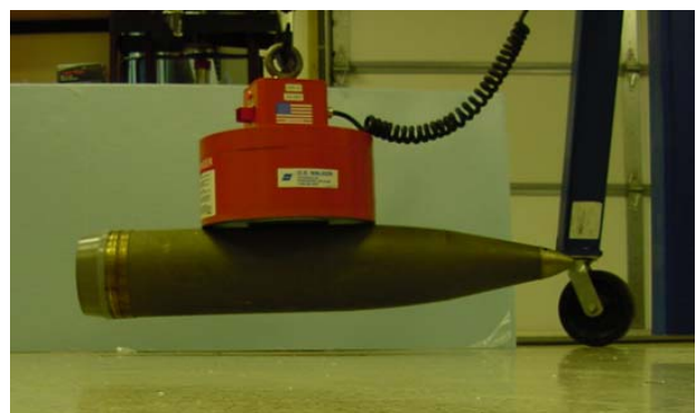
Figure 2-18. This image shows the Walker CER 12 electromagnet capturing a 155 mm projectile.
