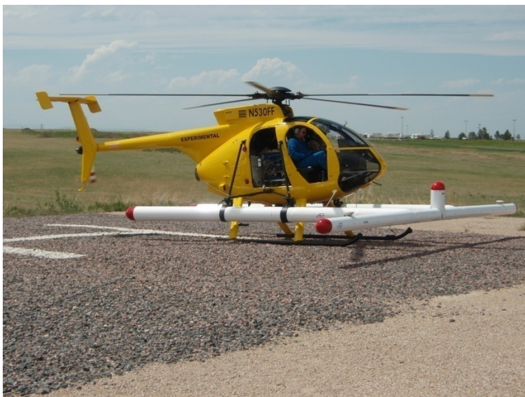
Figure 1. SKY next generation HeliMag system. The sensor boom holds a linear array of 13 magnetometers spaced 0.75m apart. A 14th sensor is temporarily mounted above the middle sensor to provide measured vertical gradient test data. The system is operated with an 'Experimental' category airworthiness certification.
