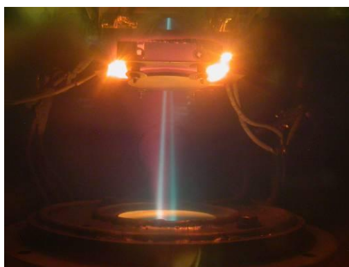
Figure 4: The split e-beam can be seen as well as part of the heating element used to heat the 4340 steel substrates.
