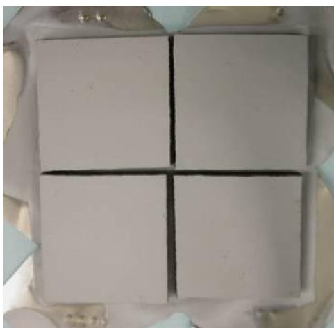
Figure 8: Representative 1"x1" 4340 steel substrates coated with a Zn-Ni-Co alloy.
