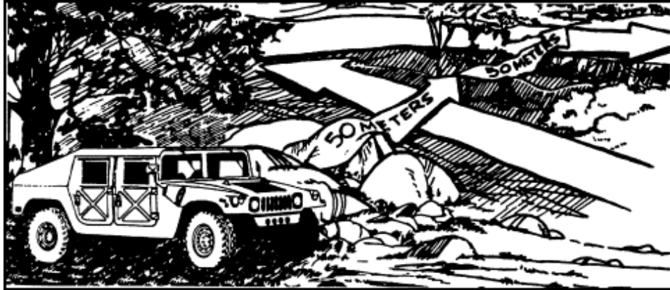
Figure 3. Slow-Scan (50-Meter) Technique.
