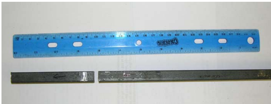
Figure 11. Low carbon steel bar from which samples were obtained.
