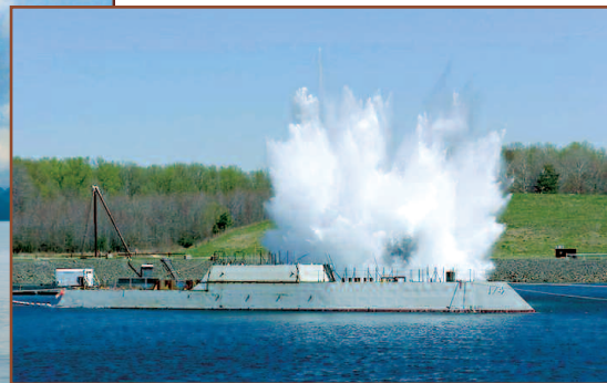
Left: Artistic rendering of the DDG 1000 in action, along with the program's logo. Above, a DDG 1000 model undergoing structural integrity testing. Media provide by Robert Wunderlick, NSWC Carderock Division.
