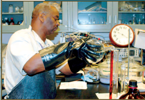
Above: Research scientist Norris Lindsey performs susceptibility testing on aluminum in a high-temperature, high-acidity environment. Temperature in the test was set at about 170 degrees Fahrenheit, with a pH of between 1.0 and 2.0.
