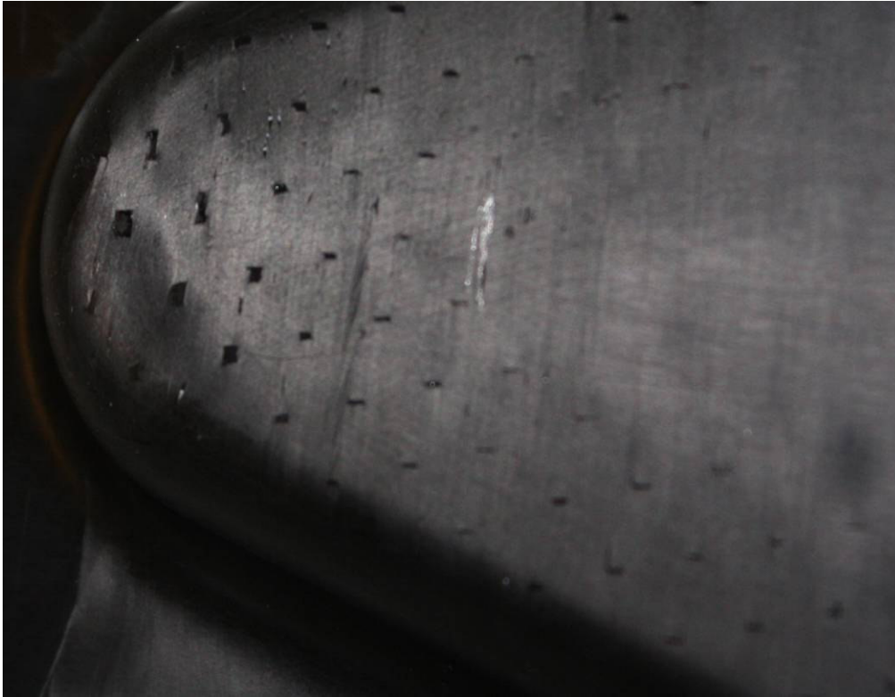
Fig. 7. Nose of Radome. Notice the gaps created by stretching. The stretching cuts were made only locally in the corners.
