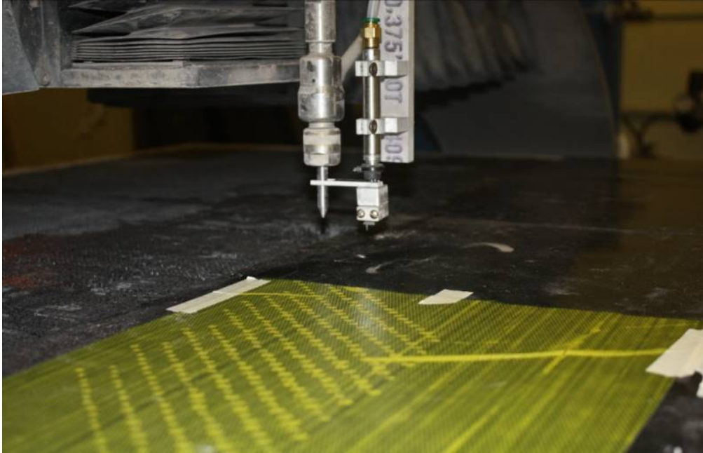
Fig.2. Cutting the prepreg using a pneumatic CNC cutter, made for this project by mounting a razor blade and pneumatic cylinder to a CNC waterjet cutter.
