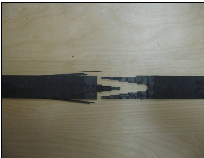
Fig. 4. Tensile specimen after failure (Pattern 5), clearly showing how the fracture followed the cuts.
