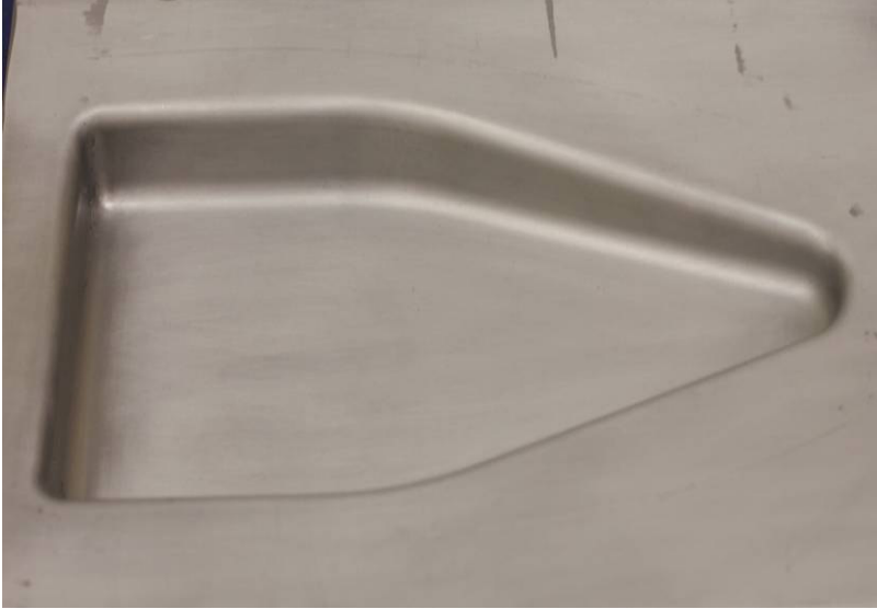
Fig. 5. Supersonic Radome Mold
