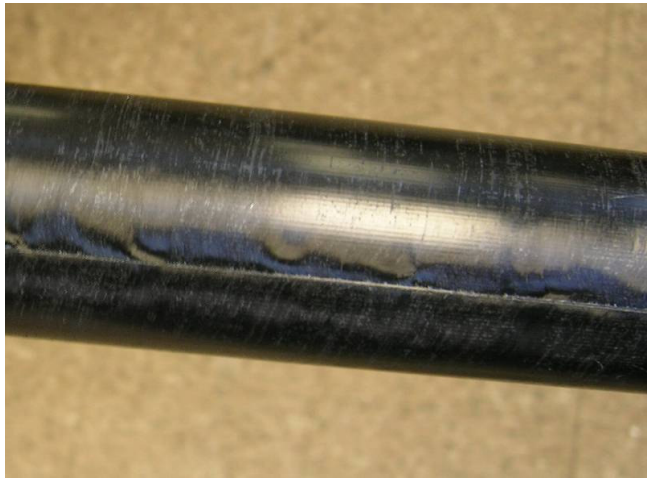
Fig. 9. Tubes wound with conventional prepreg on slightly oversized mandrels, showing fiber waviness (left) and an internal bulge (right)
