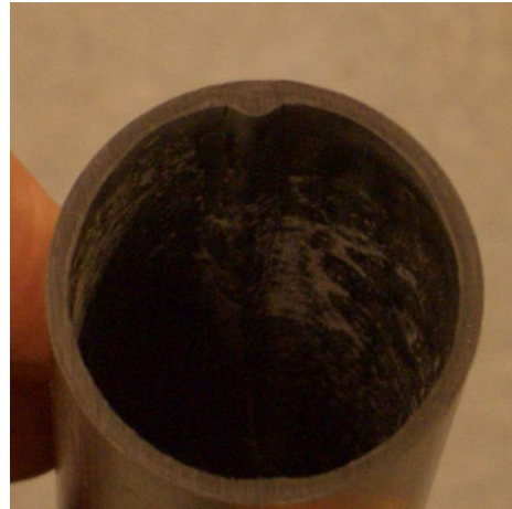
Fig. 9. Tubes wound with conventional prepreg on slightly oversized mandrels, showing fiber waviness (left) and an internal bulge (right)
