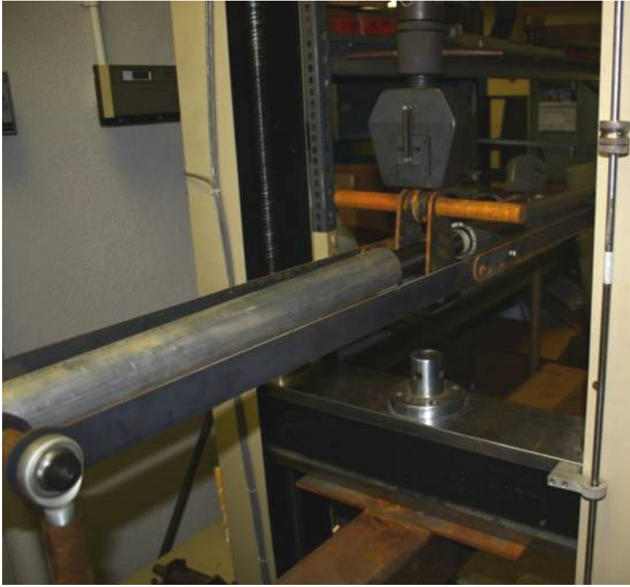
Fig. 11. Three point bend test of carbon fiber tube.
