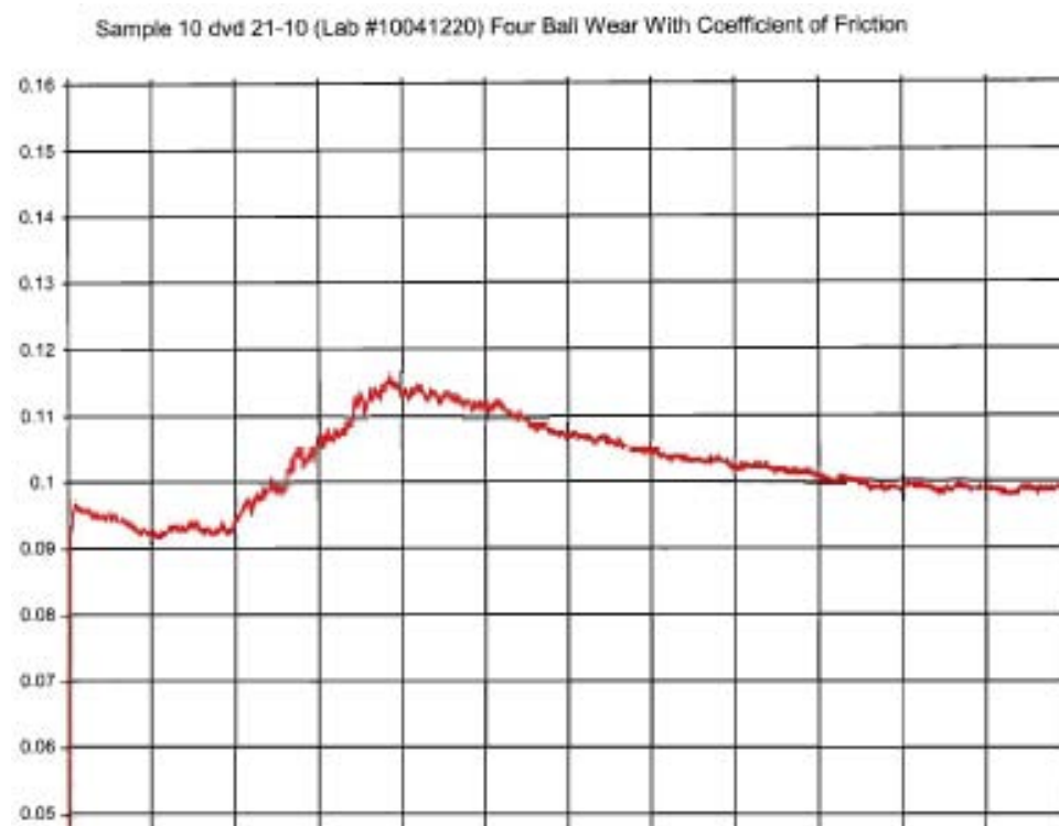
Figure B.10. Four ball test Coefficient of friction of Motor Oil “B” Formula Complete minus MoS 2 (without friction modifier additive) with W 2 nanoparticle
