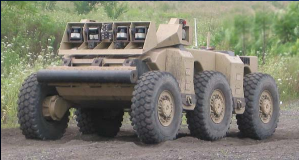
Crusher with sensors
