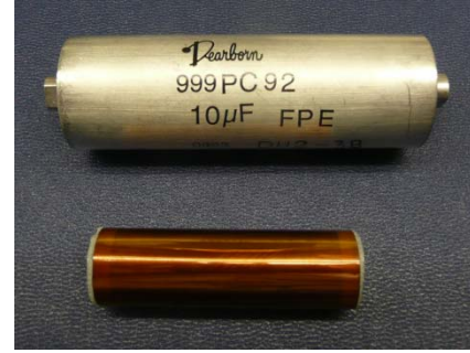
Figure 6: Pictorial view of the 10 \mu\text{F} FPE capacitors (packaged and unpackaged)
