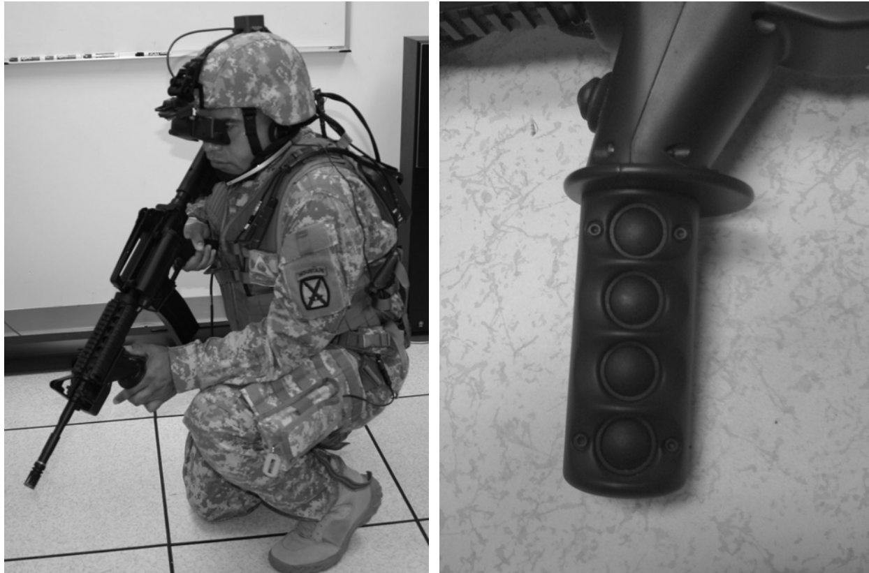
Figure 2. U.S. Army Soldier wearing the ExpeditionDI wearable simulator interface (left). The front handgrip controls from the simulated M4A1 rifle (right).
