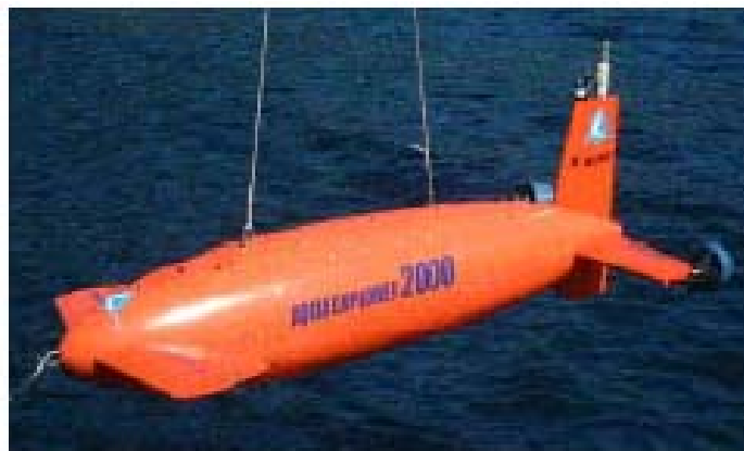
Fig. 3. AUV “Aqua Explorer” for submarine cable inspection (KDDI & MES).
