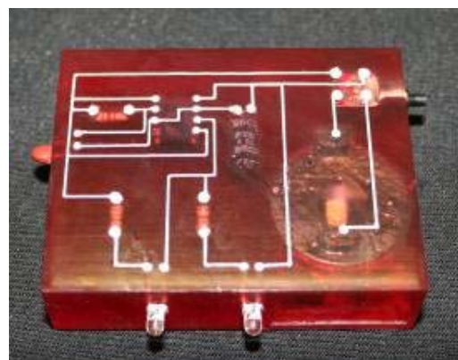
Figure 1. LM555 temperature circuit fabricated using the hybrid SL/DW setup.
