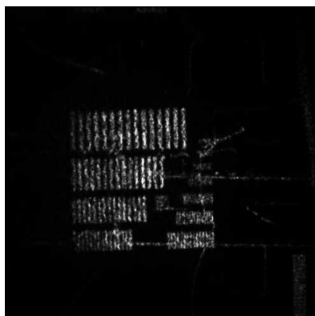
Fig. 4: Images of the entire resolution test chart inside a solution of polystyrene spheres at OD = 5 . a) without the OKE gate , and b) with the OKE gate. The images are of the same chart but were not acquired at the same scale.
