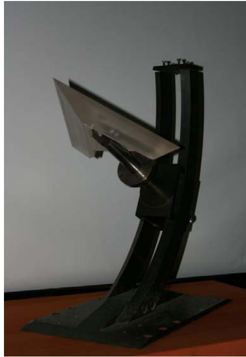
Figure 9 Photo of the delta-wing installed on the pylon
