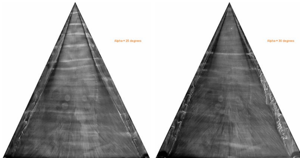
Figure 33 Oil-flow visualization on the leeward side of the delta-wing for various angle of attack ( U_\infty = 12 m/s)
