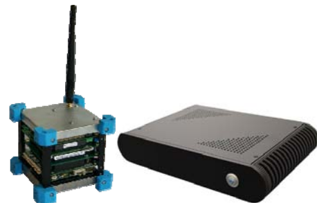
Figure 3: Boeing Mobile Routers: miniaturized (airborne) and standard (ground) versions
