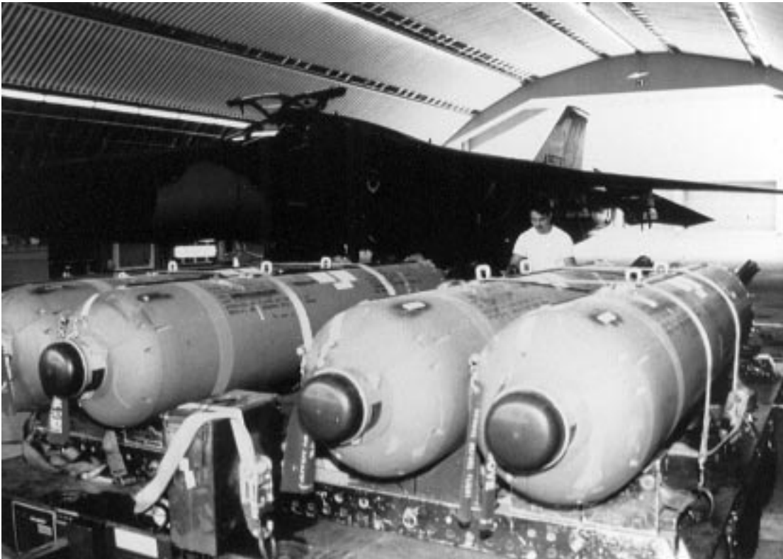
US air forces are amply equipped with cluster bombs loaded with a wide variety of submunitions and mines. Shown here are standard dispensers ready for loading onto an F-111 in the Gulf War. They often come with proximity fuzes that open the dispenser at some altitude to release a host of small submunitions over a wide area—so many, in fact, that even a very small dud rate can leave a dangerous residue. This sometimes leads both the public and the media to oppose their use. (Photo courtesy of Col Mason Carpenter, USAF)
