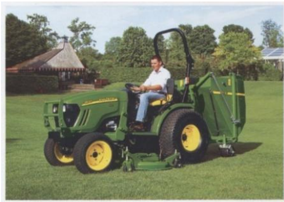
Above: John Deere 2520 Compact with cutter, catcher, and hydraulic package.
