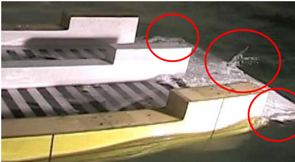
Figure 24. Side View of Water Slapping On Stern Extension, Sea State 4
