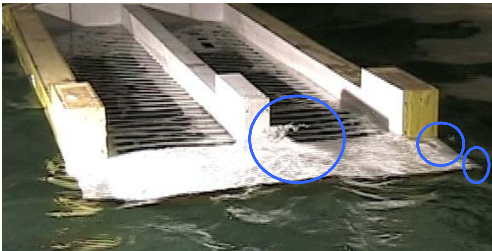
Figure 25. Water Slapping On Stern Extension during Sea State 4
