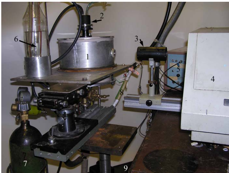
Fig.10. The general view of the experimental installation. 1 – experimental cell, 2 – cell for experimental gas mix, 3 – quartz lens, 4 – monochromator, 5 – impulse current generator for plastic film destroy, 6 – device for mix preparing, 7 – gas balloon, 8 – cable for e-gun feeding, 9 – vacuum pump.
