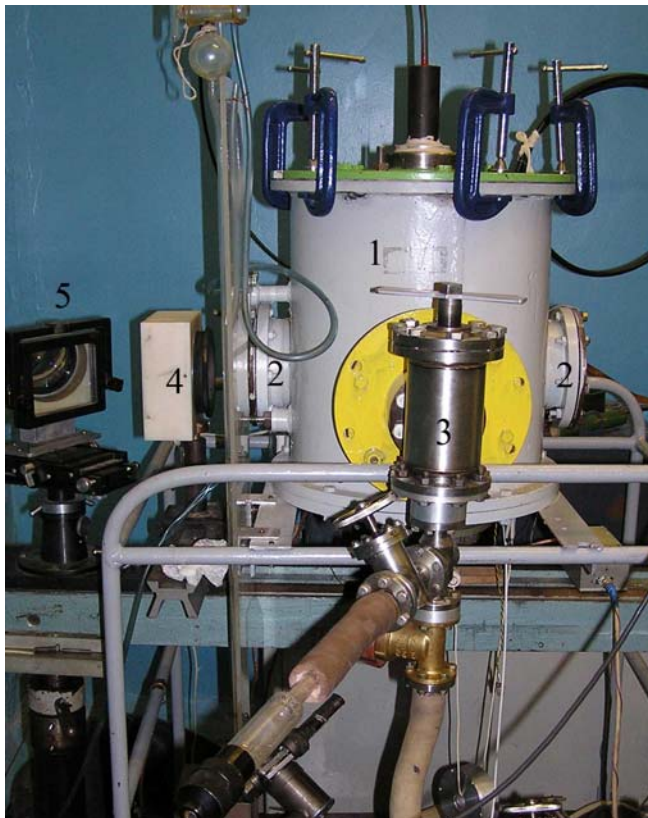
Fig. 24. Picture of the facility. 1 – body, 2 – units of optical windows fastening, 3 – vacuum valve, 4 – objective lens, 5 – turn mirror.
