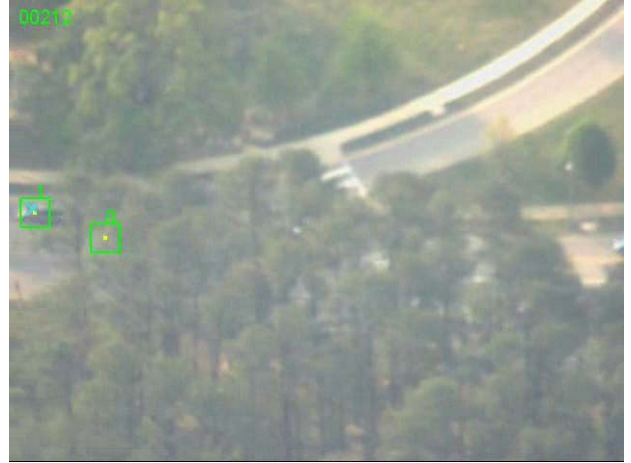
D: The reappearing target is detected by the VP and the MHT creates two hypotheses that represent two possible alternatives: the new detection belongs to the target, or the new detection belongs to another vehicle.
