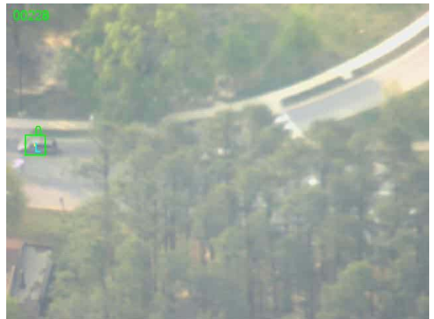
F: A highly confident CID response induces the pruning of the least likely hypothesis by MHT. In this case, the hypothesis that claims that “this is the same target” is maintained while the alternative hypothesis that claims that “this is another target” is removed.
