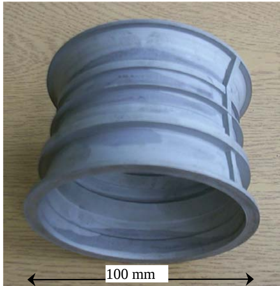
Figure 7: Showing the net-shape-HIPed mini Ti64 casing.
