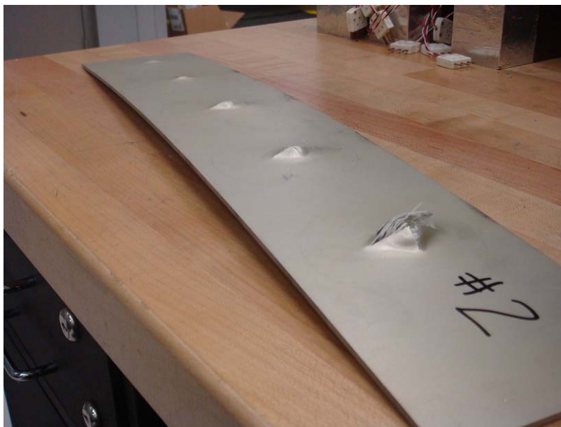
Figure 18. Reverse Side Dimpling and Cracking on GLARE as a Function of Impact Energy Progression (20, 40, 60, 80, and 100 Joules) with Constant Mass
