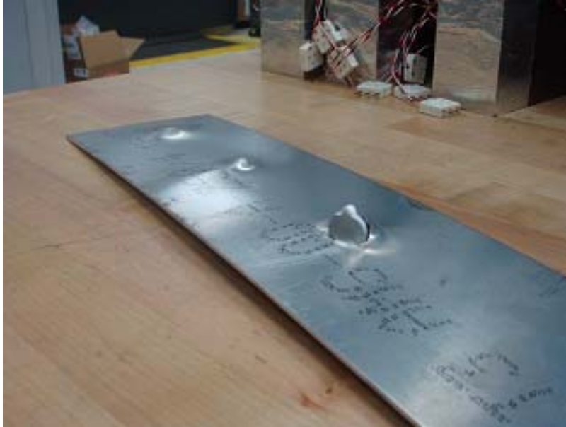
Figure 19. Reverse Side Dimpling of 2024-T3 Aluminum as a Function of Increasing Impact Energy Progression (20, 40, and 60 Joules) with Constant Mass
