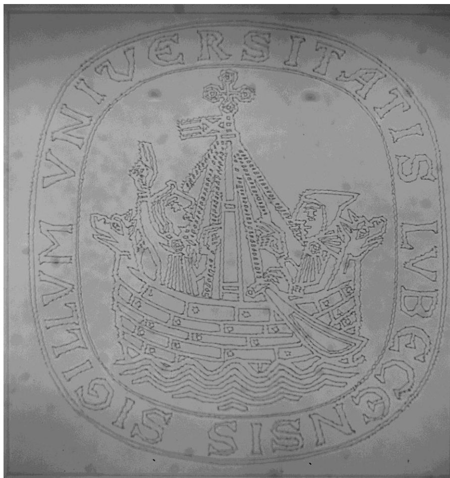
Figure 7.4 Logo of the University of Luebeck composed of micro-cavities created inside a microscope glass slide. Image height: 4 mm.
