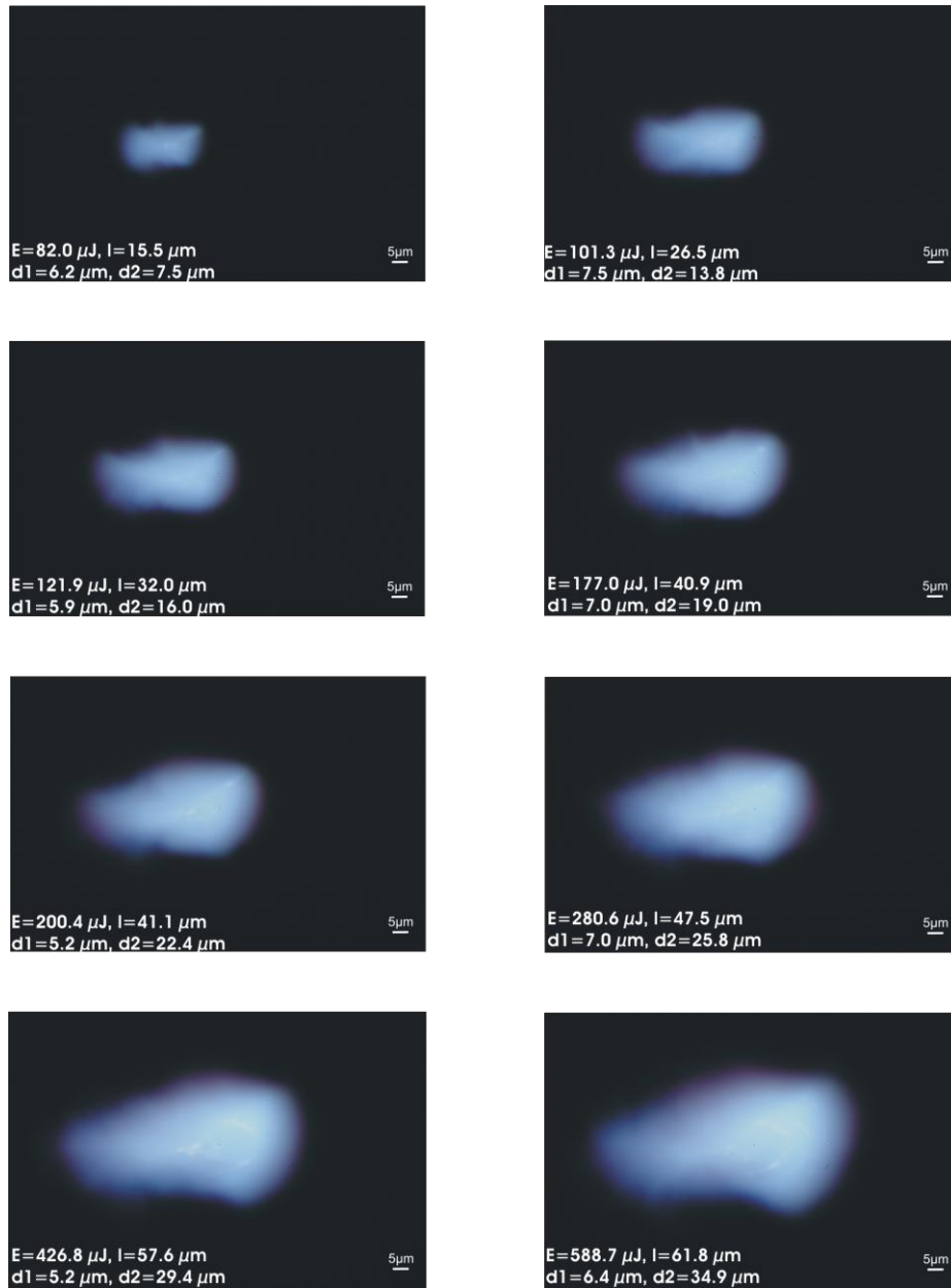
Figure 11.21 Photos of luminescent plasmas produced by seeded 11-ns laser pulses with 1064 nm wavelength focused at NA = 0.8. The values of the pulse energy, the plasma length and diameters are indicated on each frame. The light is incident from the right.
