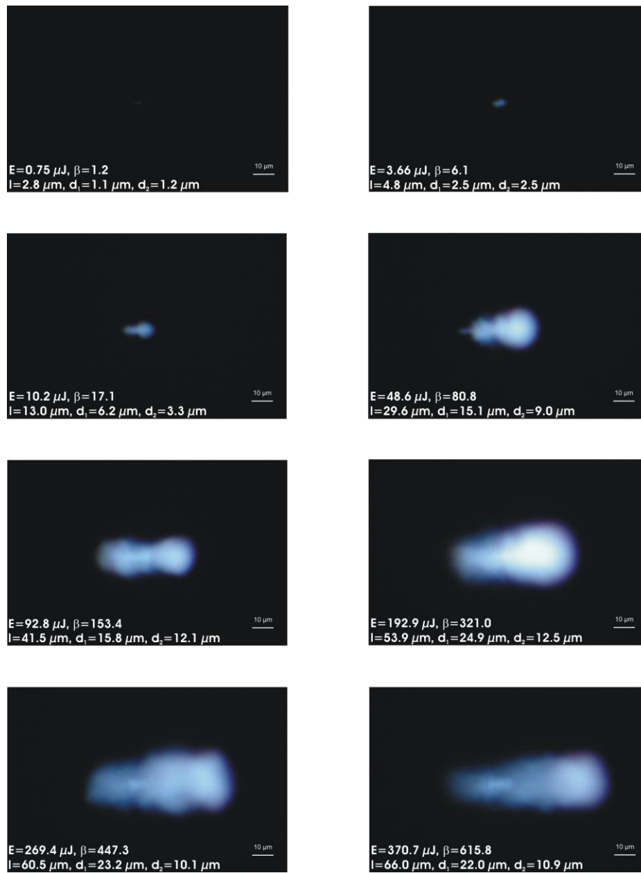
Figure 11.25 Photos of luminescent plasmas produced by unseeded 6.8-ns laser pulses with 355 nm wavelength focused at \text{NA} = 0.8 . The values of the pulse energy E , normalized energy \beta = E/E_{\text{th}} , plasma length and diameter are given on each frame. The laser light is incident from the right. The white bar represents 10 \mu\text{m} .
