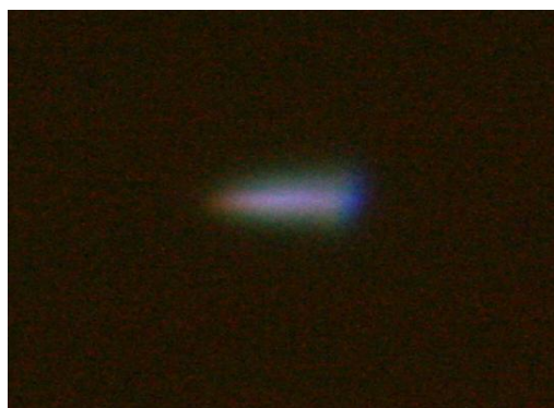
Figure 11.16 Photos of luminescent plasmas produced by 352-fs laser pulses with 1040 nm wavelength focused at NA = 0.8 . The values of the pulse energy E , normalized energy \beta = E/E_{th} , and plasma length are given below each frame. The laser light is incident from the right. The white bar represents 5 \text{ }\mu\text{m} . The photographs are integrated over 70 laser pulses, the camera Canon EOS 5D was set to ISO 3200 and auto white balance.
