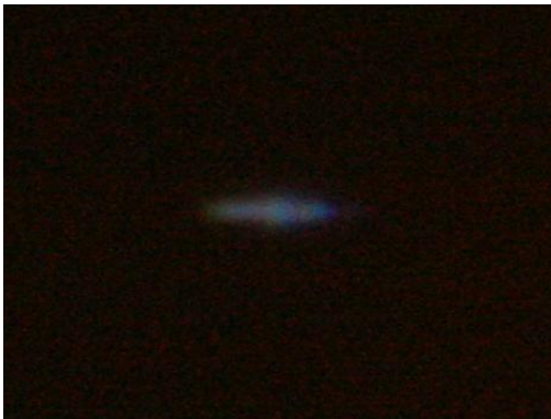
Figure 11.19 Photos of luminescent plasmas produced by 280-fs laser pulses with 347 nm wavelength focused at NA = 0.8 . The values of the pulse energy E , normalized energy \beta = E/E_{th} , and plasma length are given below each frame. The laser light is incident from the right. The white bar represents 5 \mu\text{m} . The photographs are integrated over 70 laser pulses, the camera Canon EOS 5D was set to ISO 3200 and auto white balance.
