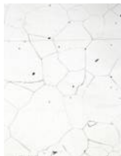
Figure 4. Section in a part of stainless steel after debinding and sintering .
