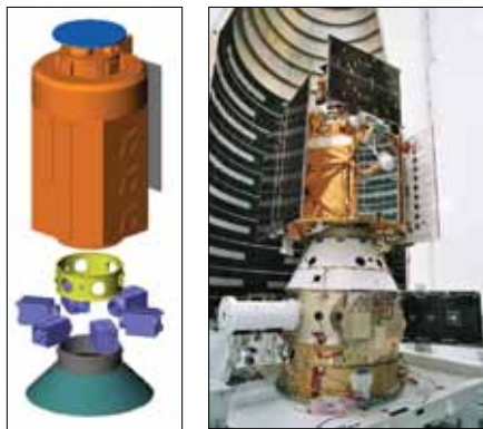
Figure 2 and 2a. Generic EELV ESPA configuration; ESPA first flight configuration on STP-1 Launch, 9 March 2007.
