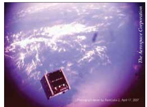
Figure 3. Cal Poly CubeSat CP-4 photographed by AeroCube-2 (launched 17 April 2007 as secondary payloads on a Russian Dnepr launcher).
