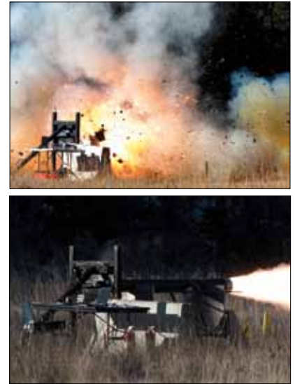
Figures 2 and 2a. FalconLAUNCH-6 explosion and FL-8 successful test.
