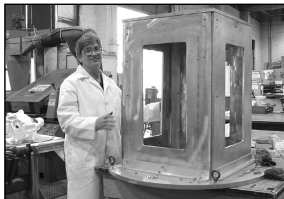
Machine Shop – fabricating radar pedestal for shipboard operation
