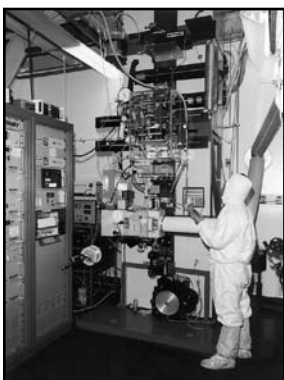
Fiber Fabrication Facility for Nonoxide and Specialty Glasses. Unique state-of-the-art draw tower used for fabricating infrared transmitting fiber from specialty glasses under controlled atmospheres using NRL-invented preform and double crucible processes.
