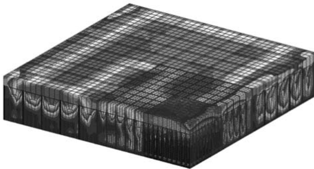
Wavelength Scaled Array: An Ultra-Wideband Array Concept providing constant beamwidth across 8:1 bandwidth; designed by NRL developed Domain Decomposition Algorithm.
