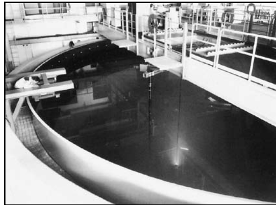
Structural acoustic studies in the one-million-gallon Acoustic Holographic Pool Facility
