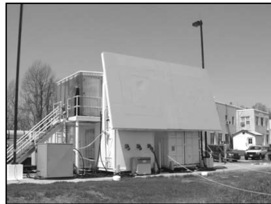
The Advanced Multifunction RF Concept (AMRFC) test-bed as a proof-of-principle demonstration system capable of simultaneously transmitting and receiving multiple beams from common transmit and receive array antennas for radar, electronic warfare, and communications.
