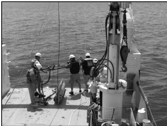
The acoustic source-receiver array (ASRA) contains twelve sources/receivers. The purpose is to conduct multiple-input multiple-output (MIMO) underwater acoustic communications experiments.
