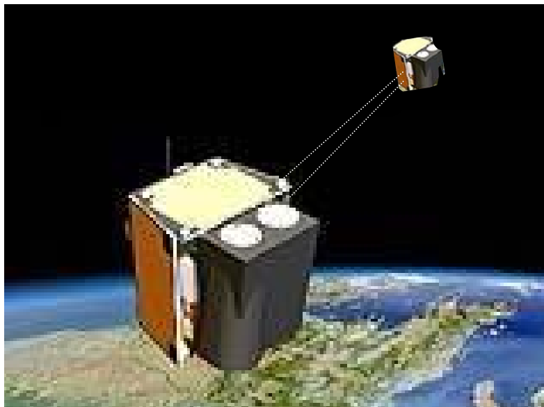
Figure 1. Droplet Stream Propulsion Concept in which Momentum is Exchanged Between Satellites Creating a Continuous Displacement Force that Maintains separation from the Reference Orbit Centerline.
