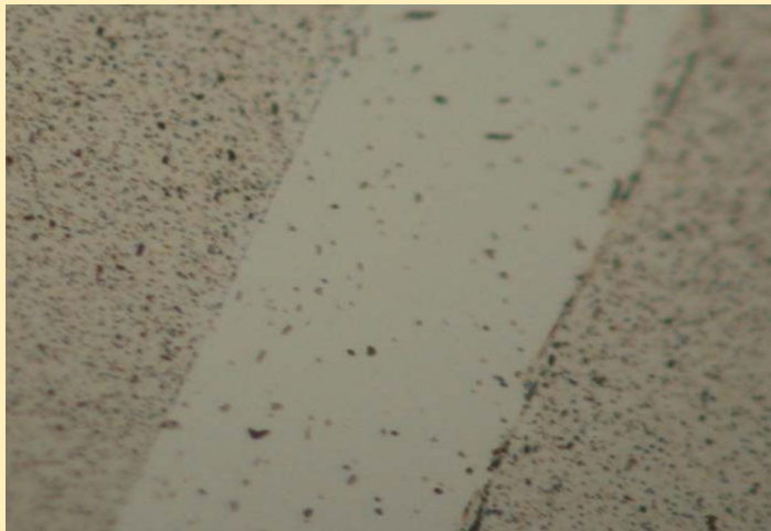
Nano grained 5083 Al laminate with 1100 Al inter-layer
