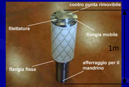
MANDREL FOR THE PROTOTYPE PRODUCTION USING THE FILAMENT WINDING
