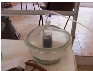
Figure 3.3.1: degassing phase of the resin employed to the manufacturing of micro and nanostructured composite samples by direct Stereo Lithography
