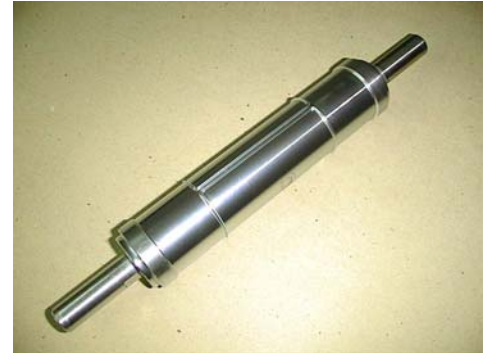
Figure 13: Laser consolidated CPM-9V rotary cutting die after final sharpening.
