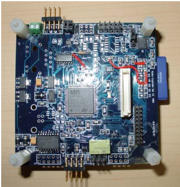
Figure 2: Completed CPU (left) and controller (right) boards for the Drifting Profiler. These boards will also be used as agent controllers for the DRONE mobile distributed sensor platforms, and are designed to communicate with the fixed wireless sensor network.
