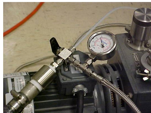
Figure 48. RIGEX MGSE_4 User control gage and valve
