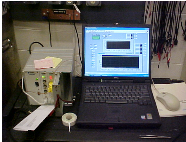
Figure 44. Data Acquisition System Running Lab view 6.0
