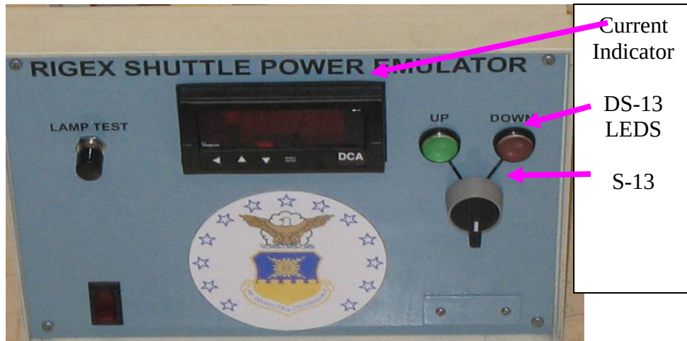
Figure H.2 RIGEX Emulator (Front)- User Interface
