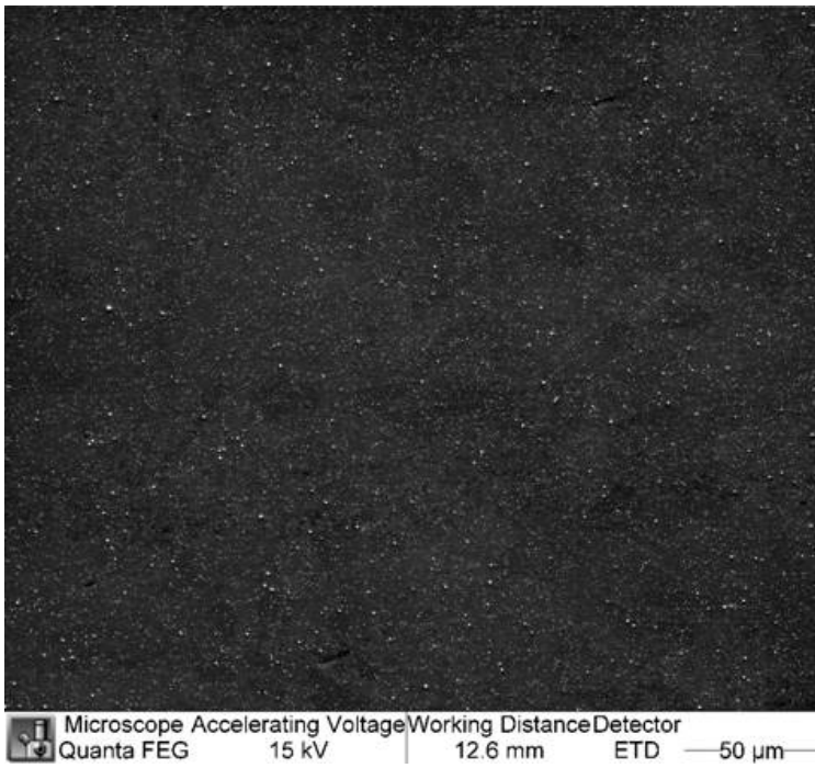
Figure 4: Secondary electron micrograph of the platinum coating used for DIC
