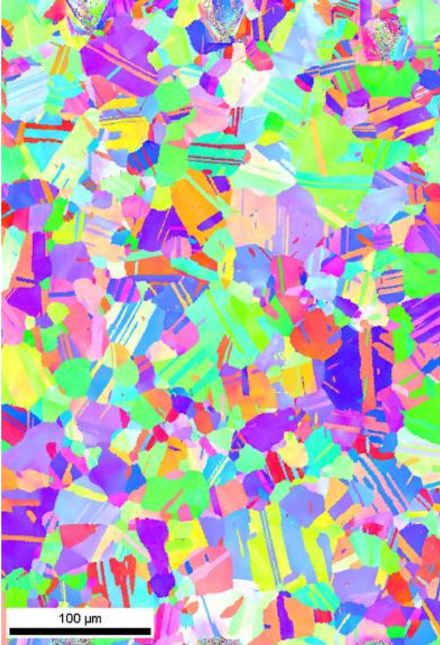
Figure 8: Inverse pole figure showing grain orientation of the deformed area
