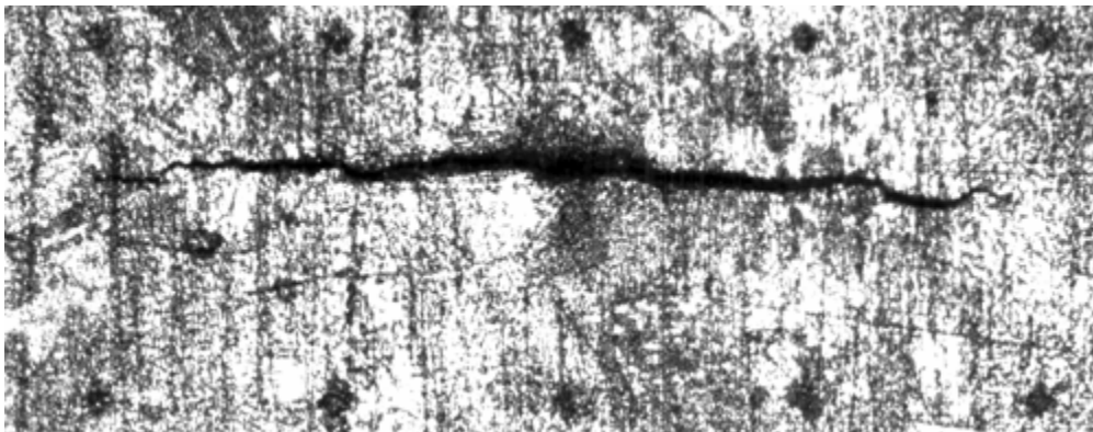
Figure x1: Optical image of fatigue crack polished and etched for DIC and marked for combining displacement and EBSD results.
