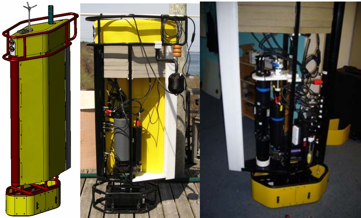
Figure 1. The AMP-ES100 profiler. Left panel shows a drawing of the profiler with the protective yellow skins, top cap and bottom battery footing installed. Middle panel shows a photograph of a profiler with one of the sides skins removed, exposing the center payload section (profiler show was delivered to NUWC, RI division). Right panel shows an AMP with both side panels removed. This profiler was used during the summer 2007 ONR OASIS experiment, and was deployed for ~2 weeks in September 2007 in 12 m off water near the Matha's Vineyard Coastal Observatory. The instrument configuration included a CTD (SBE49), a chlorophyll and backscattering sensor (WET Labs ECO FLNTUS), a single wavelength scattering sensor (WET Labs AUV-B), a current velocity sensor (Nortek Vector), and a hyperspectral absorption and attenuation meter (WET Labs ac-s).
