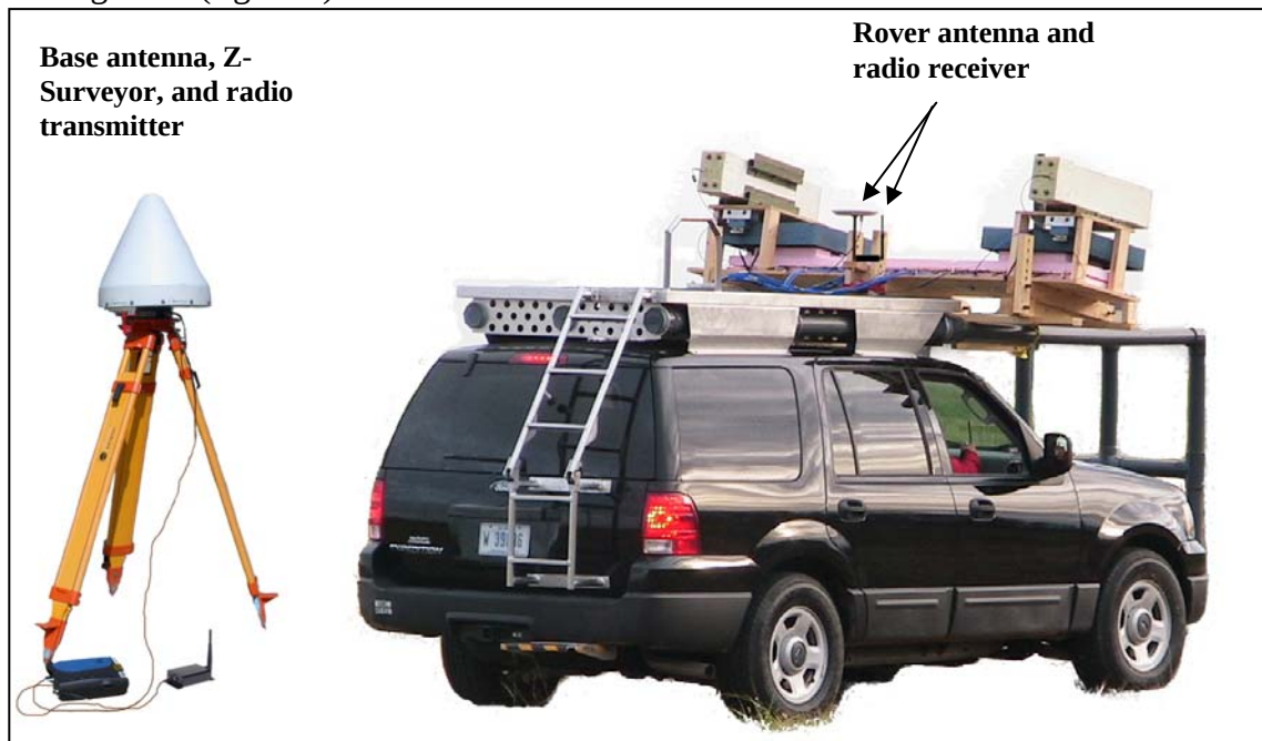
Figure 4. Example of base station setup with Z-Surveyor and NL 2400 radio transmitter (left), and rover antenna with NL 2400 radio receiver mounted on the roof of mobile platform with Z-Surveyor stored inside the vehicle (right).
