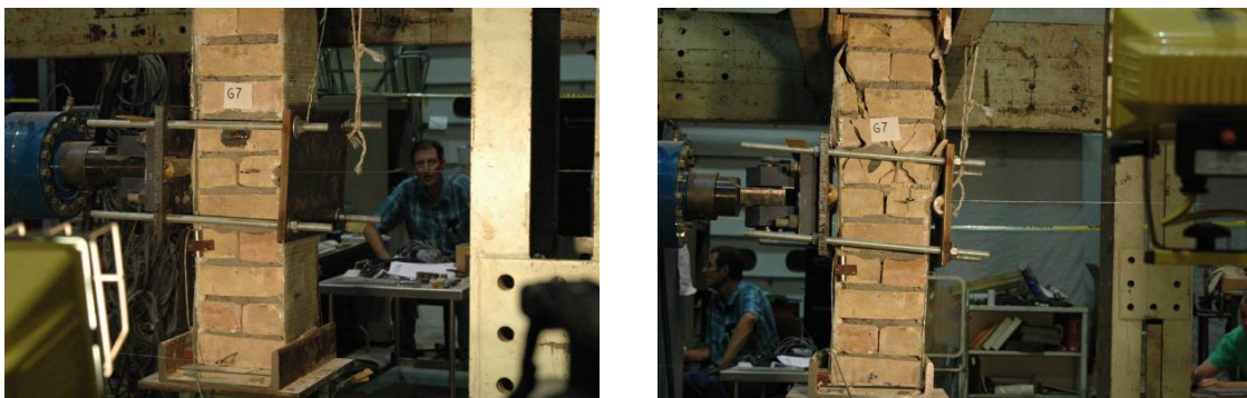
b. Specimen G7 with SikaWrap Hex, before test (left) after test (right).
