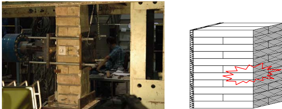
Figure 83. Specimen G8 with Sika Wrap Hex, before test (left), and sketch showing the point of failure (no picture is available) (right).
