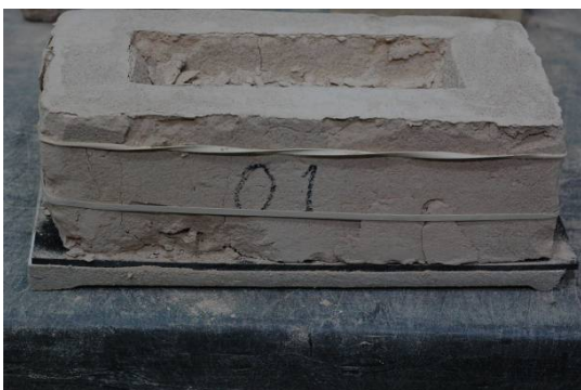
Figure 8. Single Brick from old batch # 1, no fill, after testing.
