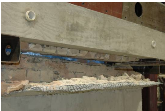
e. IP-C1 Wall after monotonic loading follow the above cyclic testing. Horizontal shear failure through the FRP.
