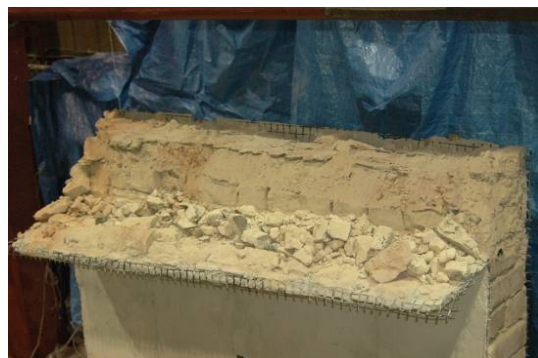
f. IP-C1 Wall after monotonic loading and after removing the unsound brick along the failure surface.
