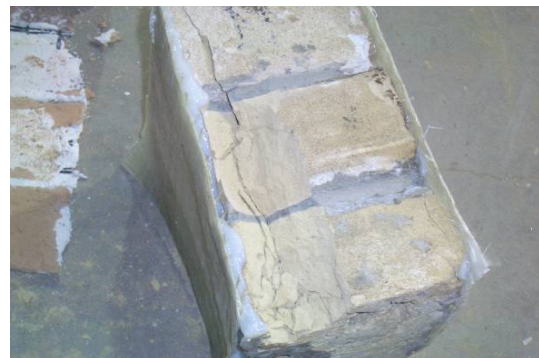
Figure 38. Prism from new batch with glass reinforcement, before (left), after (right).
