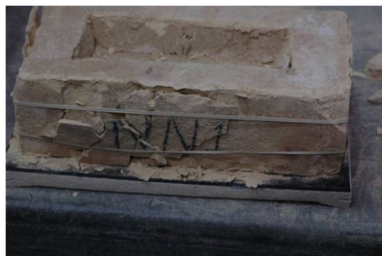
Figure 9. Single brick from new batch #1, no fill, after testing.
