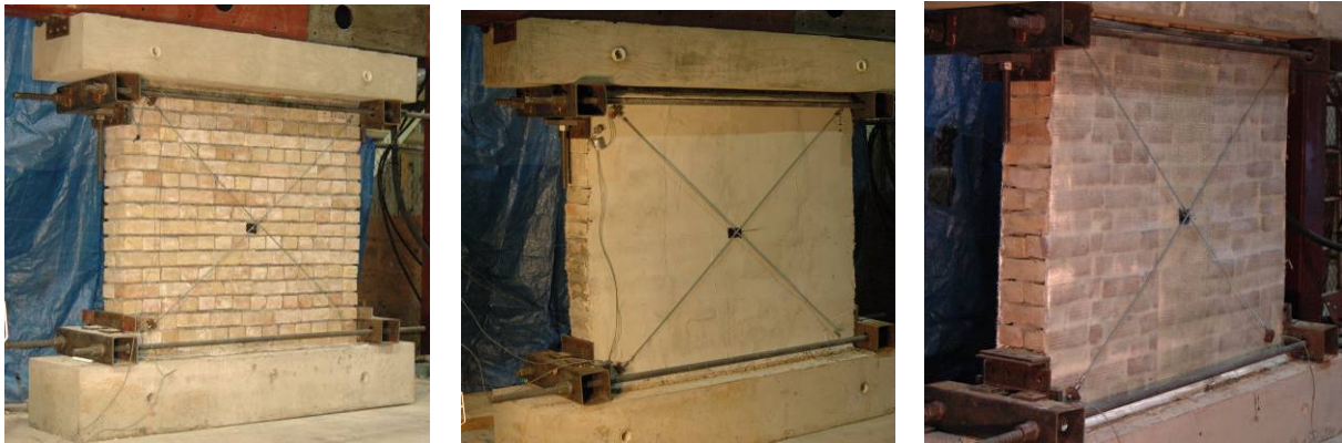
Figure 47. Bare wall (left), Saint Gobain cementitious FRP System (center), and SikaWrap FRP system (right).
