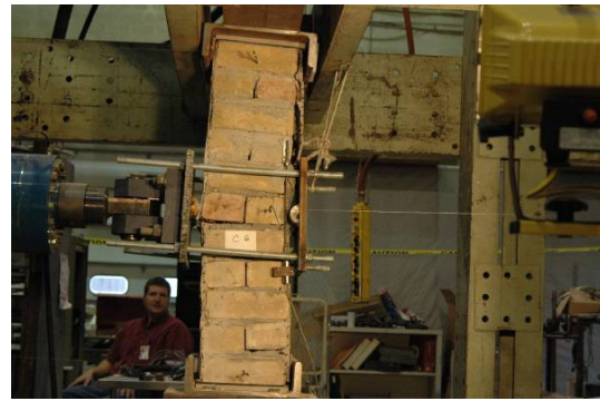
a. Saint Gobain Cement-Base Specimen C6, before test (left) after test (right).
