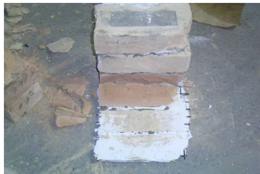
Figure 37. Prism from new batch with cementitious reinforcement, after.
