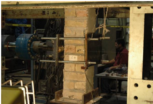
a. Saint Gobain Cement-Base Specimen C6, before test (left) after test (right).
