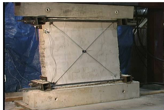
d. IP-C1 Wall during cyclic testing shown uplift as the specimen rocks (with loading tube steel beam at the corners).
