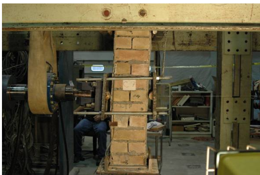
b. Saint Gobain Cement-Base Specimen C7, before test (left) after test (right).
