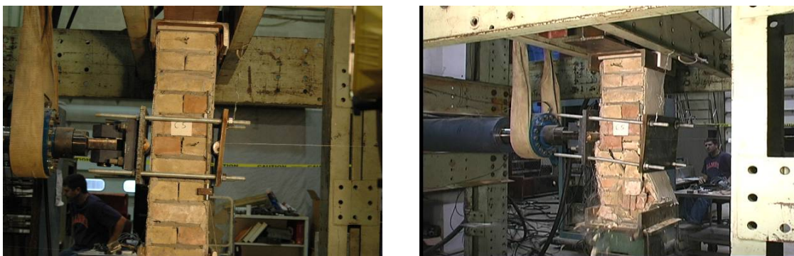
Figure 79. Saint Gobain Cement-Base Specimen C5, before test (left) after test (right).
