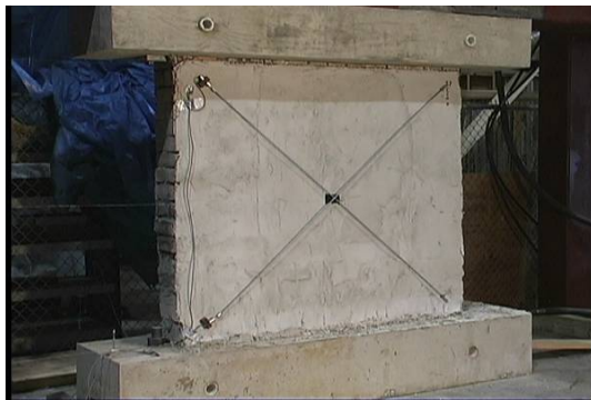
a. IP-C1 Wall prior to testing. Direct load on the header concrete beam.
