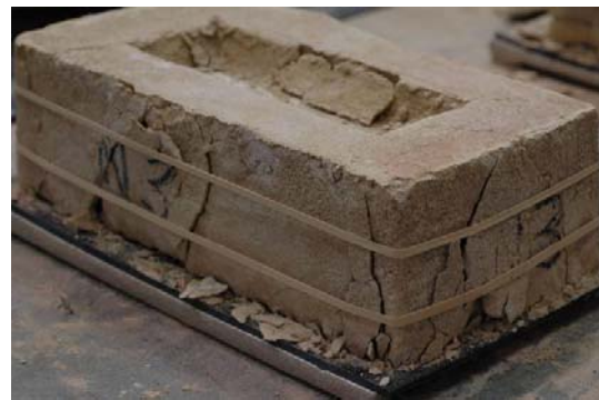
Figure 13. Single brick from new batch #3, no fill, after testing.
