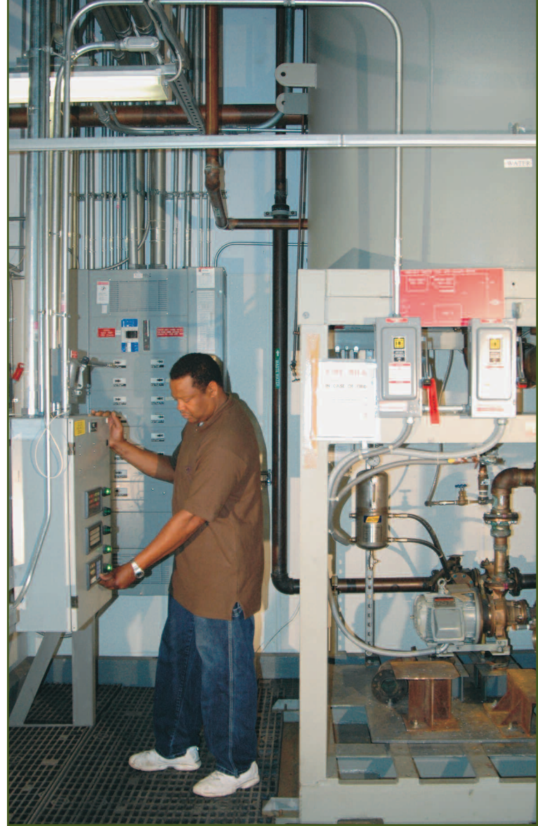
NSWCCD equipment specialist (Tom Nesbitt) conducts testing of a new commercial-off-the-shelf (COTS) shipboard sewage pump cartridge seal being installed fleetwide as a Machinery Alteration (MACHALT).
