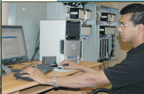
Sumit Dutta prepares to perform software testing on the LHD Improved Fuel Fill Control System at the Auxiliary System Automation Test Facility. Photo by Martin Sheehan, NSWC Carderock Division.
