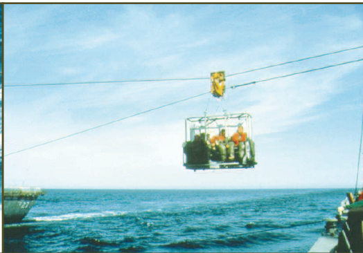
Port Hueneme Division has experimented with a six-man chair. It is feasible that a chair capable of transferring 10 personnel at a time could be used in the Sea Base mission.
