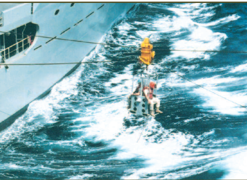
Currently, one or two personnel are transferred at a time by this tensioned wire rope system.
