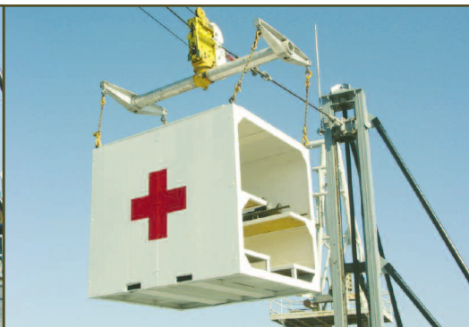
The UNREP ambulance could be used to transfer 100 patients per hour by tensioned wire rope rig.
