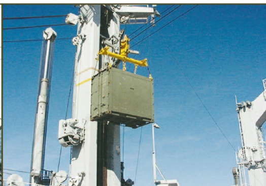
The future Heavy UNREP system with USMC QuadCon load up to 12,000 pounds.
