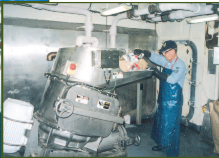
Below: The large pulper installation on USS George Washington (CVN-73). Detailed design guidance for the pulper as a solid waste management option for implementation aboard large ships is provided in the NAVSEA Design Supplement that corresponds to Naval Vessel Rules for Paper and Cardboard Waste.
