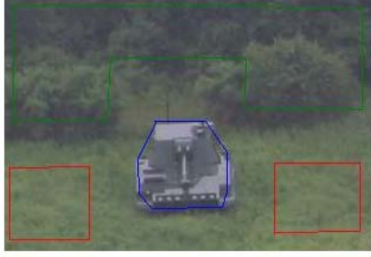
Figure 6. The test target and its natural background. The target, grass and trees regions of interest correspond to the blue, red and green boxes, respectively.
