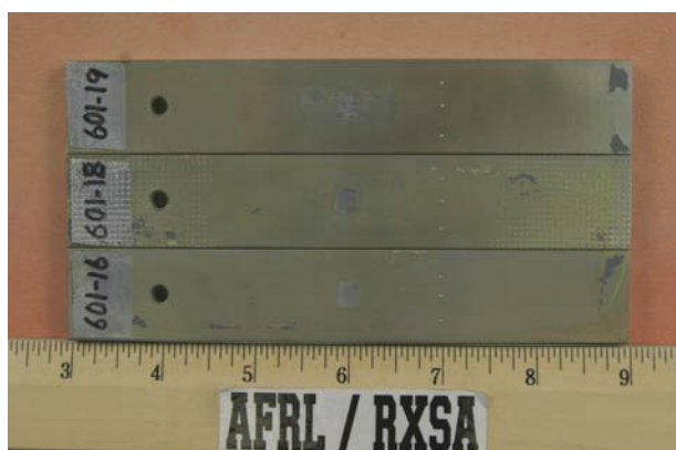
Figure 13. 2024-T3 Specimens Processed with Chemical Stripper
