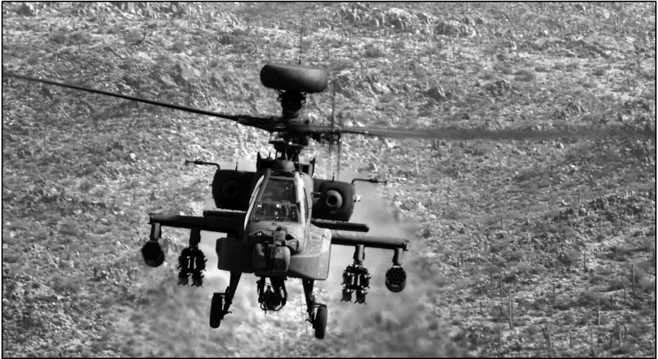
A US Army AH-64D Apache Longbow helicopter, armed with AGM-114 Hellfire air-to-ground missiles and 2.75-inch rocket pods, in flight during a test conducted at the Boeing/McDonnell Douglas facility, located near Mesa, AZ. (US Army Photo)
