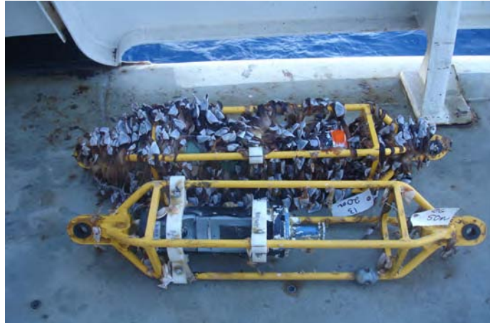
Figure 4-3a. RCM-11 recovered (back), SeaGuard crushed (foreground).
