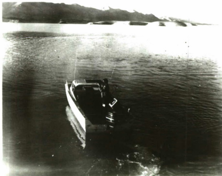
Figure 9.--View of boat with fathometer crew beginning sounding run.
