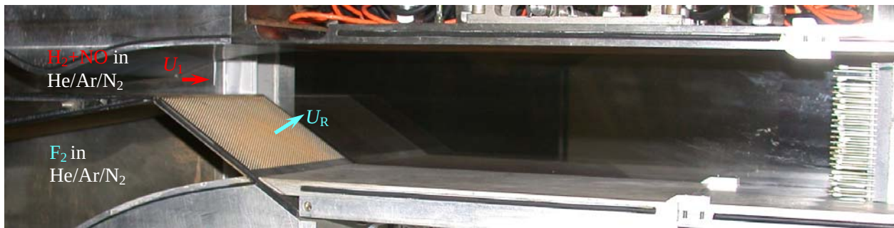
Fig. 1. The supersonic shear-layer facility expansion-ramp flow geometry
