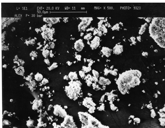
Fig. 8.4. SEM micrograph (x 500) of propellant P_01a condensed products at 30 bar.
