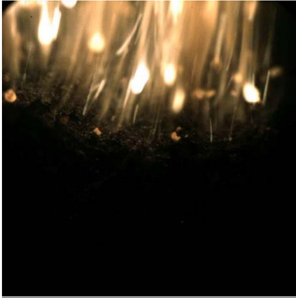
Fig. 7.5. 30 \mu\text{m} spherical micro-Al in AP/HTPB, burning at 10 bar, showing exudation aggregates over the surface and agglomeration after inflammation at some distance from the surface.
