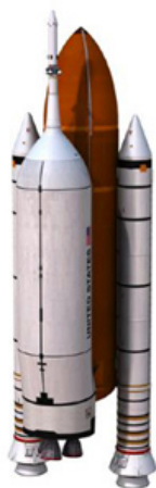
Figure 5.2.2-2. Shuttle-Derived Sidemount Launcher. Source: NASA
