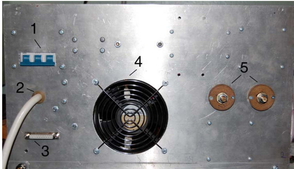
Fig. 16. Appearance of the rear panel of the experimental version of the SPS.
