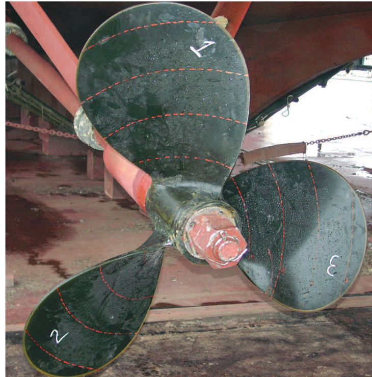
Port encapsulated propeller on YP 677. Installation is latest in series of real-world demonstrations of encapsulated propulsor performance.
