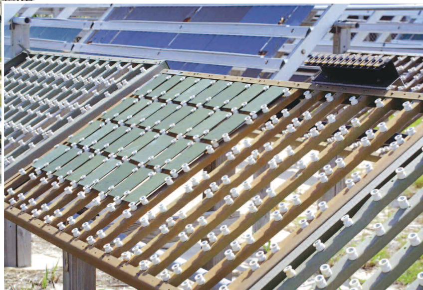
Overall view of the near-ocean test lot and of ongoing marine atmospheric exposure tests (close-up) being conducted at the LaQue Center for Corrosion Technology Kure Beach Marine Atmospheric Test Facility.
