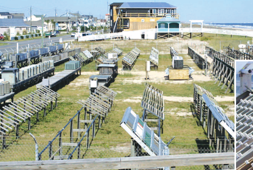
Overall view of the near-ocean test lot and of ongoing marine atmospheric exposure tests (close-up) being conducted at the LaQue Center for Corrosion Technology Kure Beach Marine Atmospheric Test Facility.
